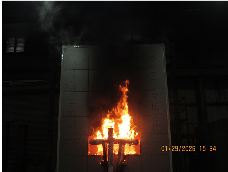
Photo No. 17 Flame tips at 7.5-ft
